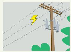
Reclosers help restore power quickly in situations where a short circuit has occurred, but the damage isn't permanent (such as a limb falling through the line). Many short circuits that occur happen like this. Customers may notice a 5-second outage when this type of short circuit occurs.
