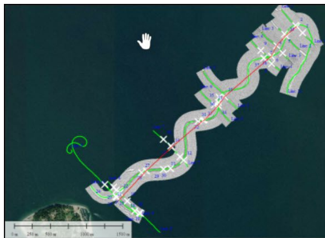
Figure 22. Magnetometer and sidescan sonar data. White marks are location of magnetic anomalies Bathymetry along entire cable route and location of existing power cable based on interpreted magnetometer and sidescan sonar data (Terrasond Ltd., 2019).
