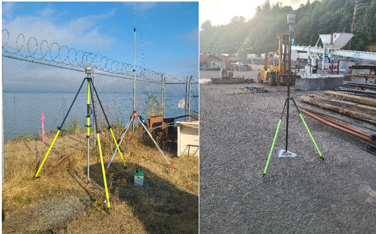
Figure 2-4. Photos of the District’s Survey Control on Port of Everett Property (rebar w/ yellow cap photo on left used for RTK and mag nail in asphalt photo on right)
