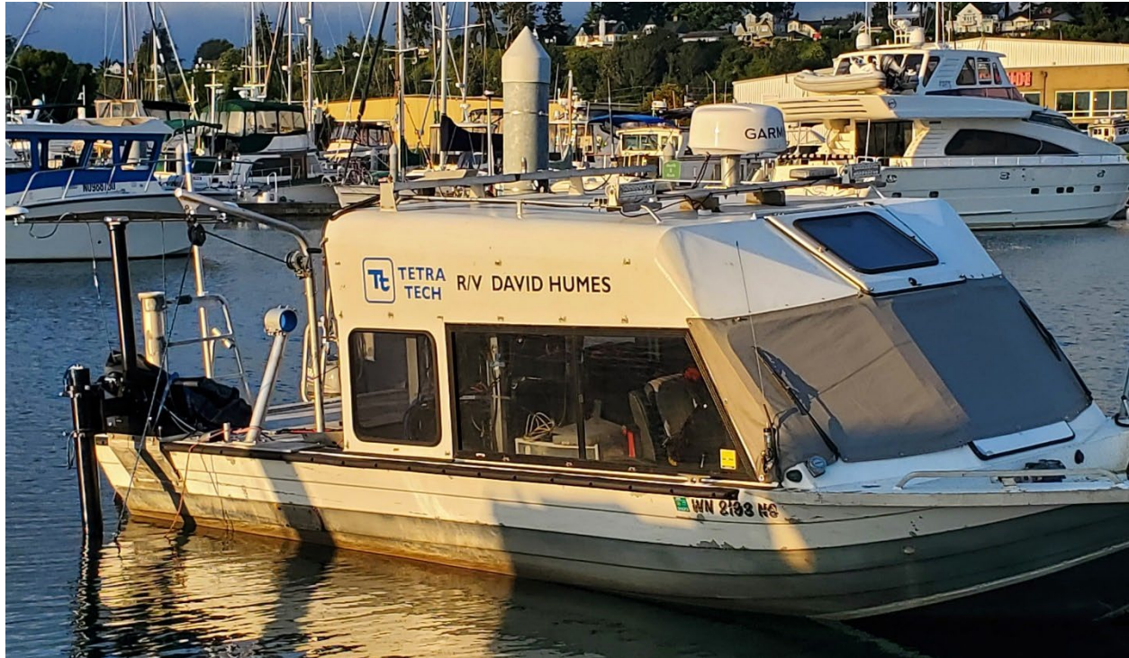
Figure 2-1. Tetra Tech Survey Vessel with R2Sonic 2026 MBE on Starboard Stern
