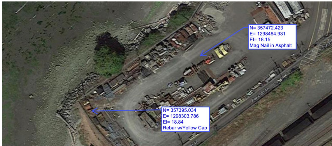
Figure 2-3. Survey Control Established at the Port of Everett by the District
