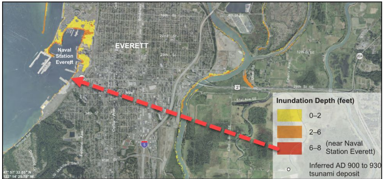
Figure 7c Inundation depth produced by magnitude 7 fault along Seattle Fault Zone (Walsh et.al., 2019)
